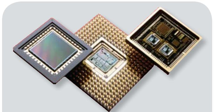
**Figure 1.** Modern components present a challenge for conformal coating, due to low standoffs and fine features.
