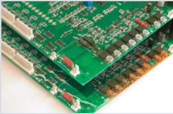
**Figure 2.** A populated PCB (bottom) shows corrosion due to insufficient protection from chemical, thermal, and electrical wear-and-tear.
