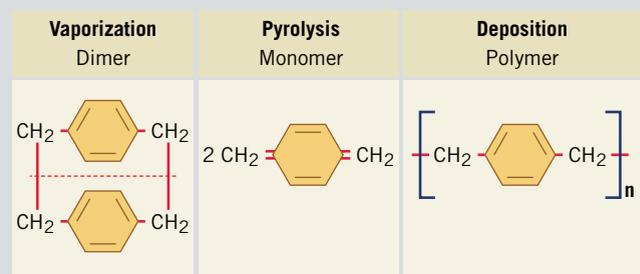
**Figure 3.** Parylene coating involves vaporizing dimer, heating the vapor to a monomer form, then depositing it as a polymer on a PCBA's surface.
