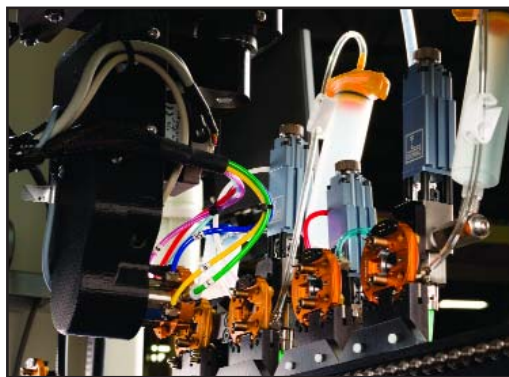
Automatic quick change (AQC) allows the use of five separate tools within a single machine.
